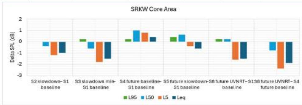
Figure 4. Table and graph showing the changes in modelled underwater noise levels from existing slowdowns and potential future vessel scenarios in Haro Strait and Boundary Pass. Table columns S4 and S5 show changes in modelled noise levels with Trans Mountain vessels relative to baseline conditions and ECHO slowdowns from 2022 (S1). (Same source as above.)
